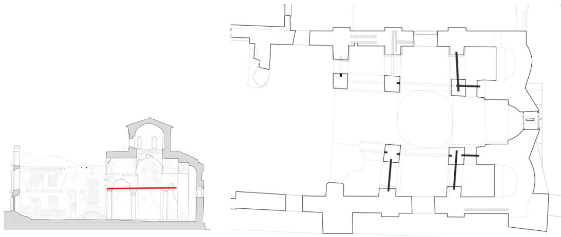
Fig. 7: Panagia Pantovasilissa, Trigleia, plan and longitudinal section showing the surveyed wooden reinforcements at the level above the columns (Mamaloukos and Kamboli 2013)
